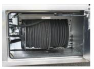
wand, delivering a high pressure stream to break up material. A self-wind reel has 75 feet of high pressure hose, while an optional hose reel has up to 350 feet of high pressure hose.
